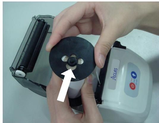
4. After installing the paper roll, reinstall the plate as the picture shows.
