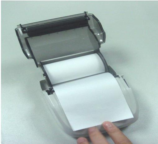
5. Place the paper roll in the slot and pull out the paper for about 3~4cm.
